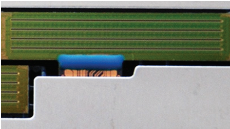
Figure 5: Detail of an HP Thermal Inkjet die
